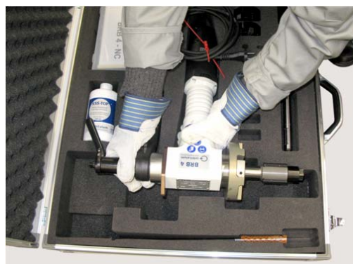
Removing the BRB from its case
